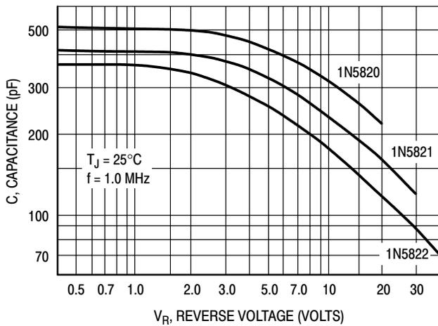
Figure 10. Typical Capacitance
