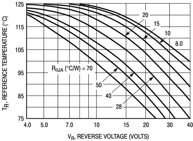
Figure 3. Maximum Reference Temperature
